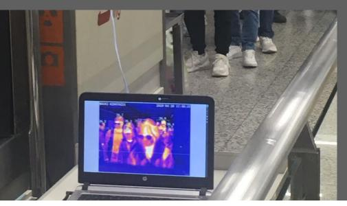
Transportation stations, including subways, railways and airports, are equipped with infrared thermometers, the system automatically detects the temperature of passengers when they pass security checkpoints. **#10**
